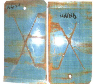
Left Panel: 2 pack liquid epoxy primer with top coat.
